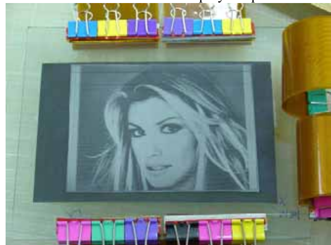
Figure 7. The image of 5.7 inch PLD panel with 320× 240 array of pixels.
