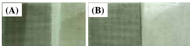
Figure 3. The tape test for CNTs adhesion ability to plastic substrates: (A) without 3-ATS treatment and (B) with 3-ATS treatment.
