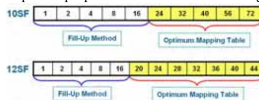
Fig. 6. The gravity centers of all 256 gray levels. 10 subfields (1-2-4-8-16-24-32-40-56-72).
