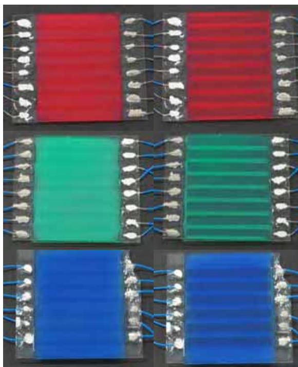
Figure 7. Demonstration photographs of pattern RGB PDLC cells switched ON (right) and OFF (left) for reflective type.
