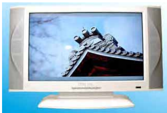
Fig. 4 Photograph of the first TFT-LCD panel (23-inch) performed by plasma beam aligned technique in the world.
