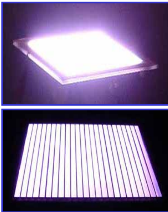
Figure 5. Discharging picture of the FFL
