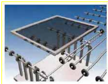
(Figure 9) Mask switching by cross rollers
