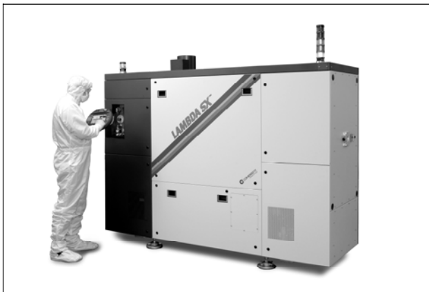
Figure 2: LAMBDA SX 315C high power excimer laser.
