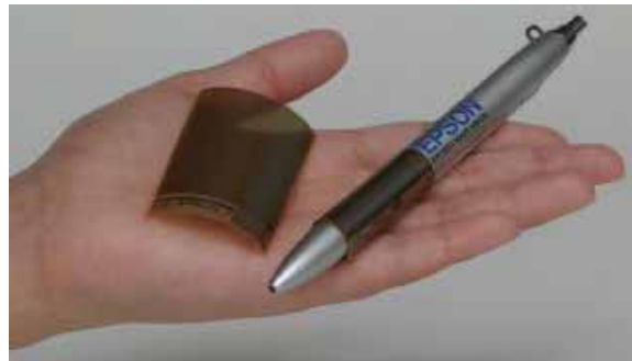
Fig. 1 Suflta polysilicon TFT devices formed on 30- \mu\text{m} -thick polyimide films
