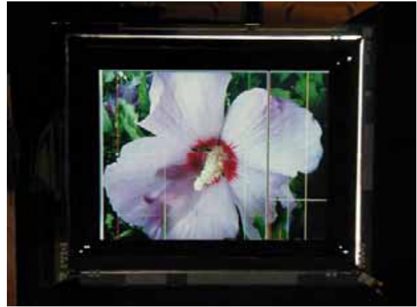
Figure 6: full color 4'' quarter VGA AMLCD addressed with display drivers and dedicated addressing system
