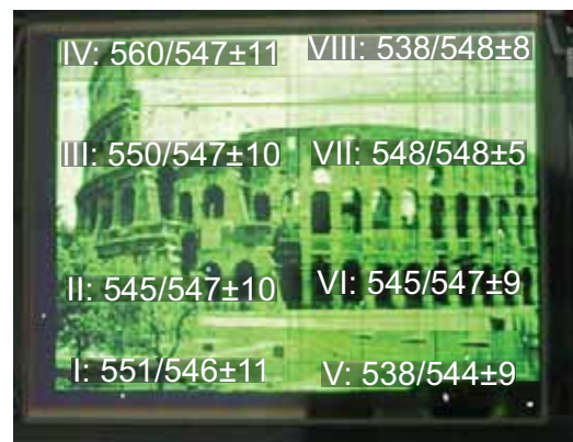
Figure 9: Monochrome green demonstrator with eight laser spots, showing energy density of the last, average and standard deviation of ten shots
