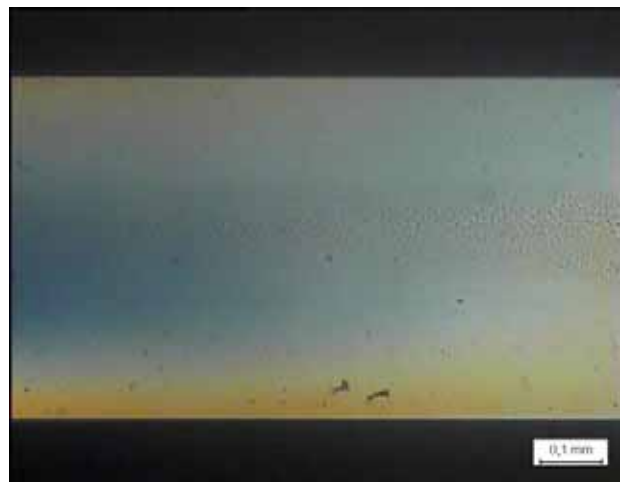
Figure 5: Laser Cut Of Glass Is Free Of Micro Cracks
