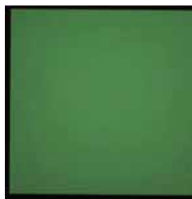
Figure 4 Picture of a 1 cm 2 OLED pixel with an 'edge seal' of 1.5 mm, after ageing more than 500 hrs 60C/90RH
