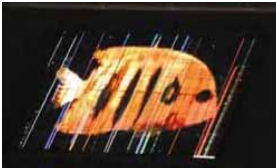
Figure 6 Full color image demonstrated on a thin film encapsulated, 100 ppi, 4" diagonal AMOLED display on steel foil.
