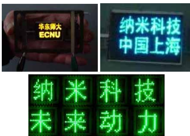
Fig. 5: Field emission display prototypes: (a) yellow; (b) blue; (c) green
