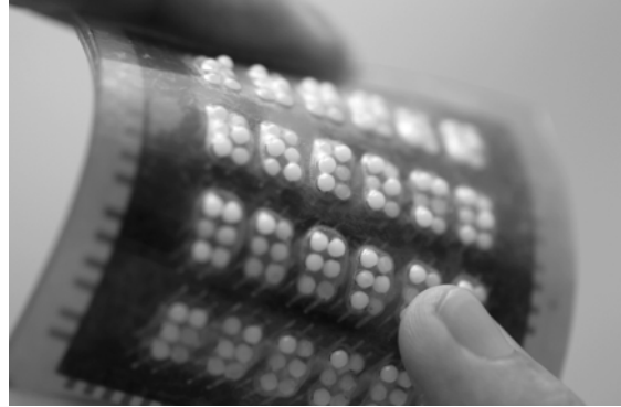
Fig. 8: An image of a pocket Braille sheet display that was manufactured on a plastic film by integrating the active matrix of organic TFTs with a plastic sheet actuator array. A hemisphere is attached to each actuator, which bends and lifts the hemisphere.
