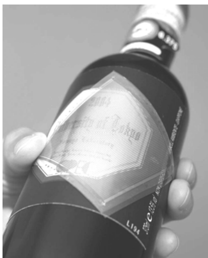
Fig. 5: An image of the manufactured large-area, flexible, and lightweight sheet image scanner consisting of organic transistors and organic photodiodes, which is placed on a business card.
