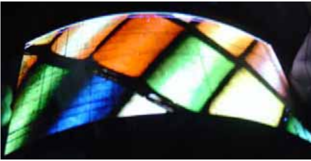
Figure 3. The display image of the 5.6 inch top emission AMOLED display on stainless steel foil emission AMOLED on stainless steel foil.
