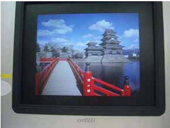
Fig. 12 The prototype of 20 inch TFT-LCD with CNT-BLU
