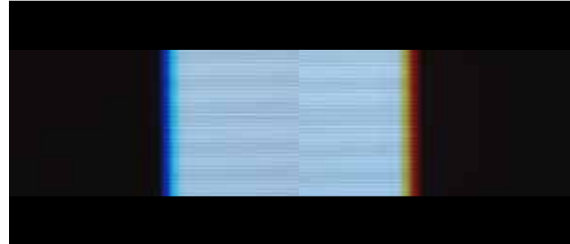
Figure 1. Example of color break up in field sequential displays
