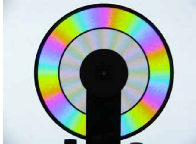
Figure 5. Example of static CBU measurement method using a wheel chopper.
