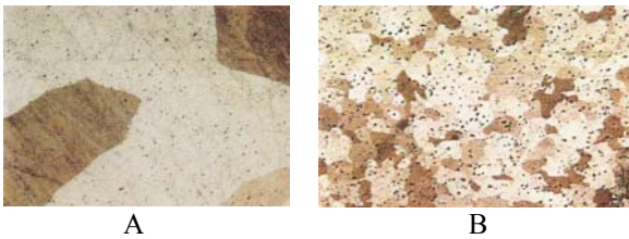
Fig. 1. Microstructure of Fe-50Co (A) and Fe- 49Co-2V (B) after sintering (magnification of 100x).
