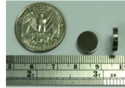
Fig. 3. The outer morphology of the Ti_{50}Cu_{28}Ni_{15}Sn_7 with 4 vol.% CNT additions after vacuum hot pressing at 723K under a pressure of 1.2GPa.
