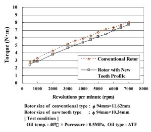
Fig. 2. Difference in Drive Torque
