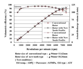
Fig. 1. Difference inVolumetric Efficiency and Actual Discharge Volume
