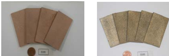
Fig. 1. Gas Pressure Infiltrated copper-diamond composite specimens, on the left are A and on the right B diamond composites.
