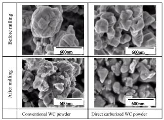
Fig. 1. Scanning electron microscope images of WC powder manufactured by conventional process and direct carburized one
