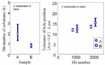
Fig. 3. Drilling performance of sample A and B (rotational speed:  $250 \text{kmin}^{-1}$ , feed :5  $\mu$ m /rev and substrate: CCL-HL832HS).
