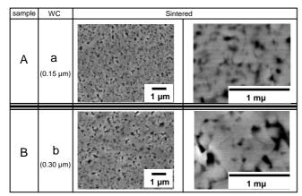
Fig. 2. Scanning electron microscope images of cemented carbides made from the WC powders of 0.15  $\mu$ m and 0.3  $\mu$ m grade.
