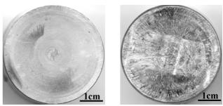
(a) Sintered composite (b) 12CrNi3A steel Fig. 3. Wear surface of the cups after the bench test.
