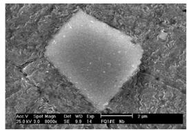
Fig. 1. A NbC particle embedded in matrix.
