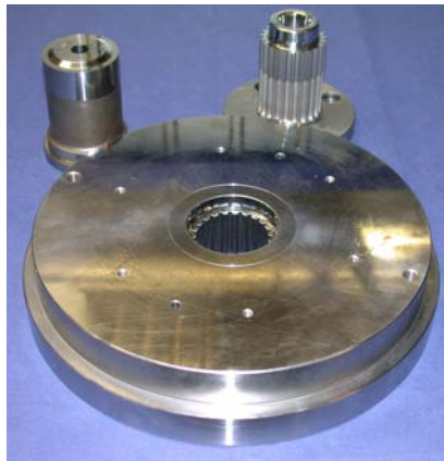
Die insert made of BÖHLER S290PM MICROCLEAN
