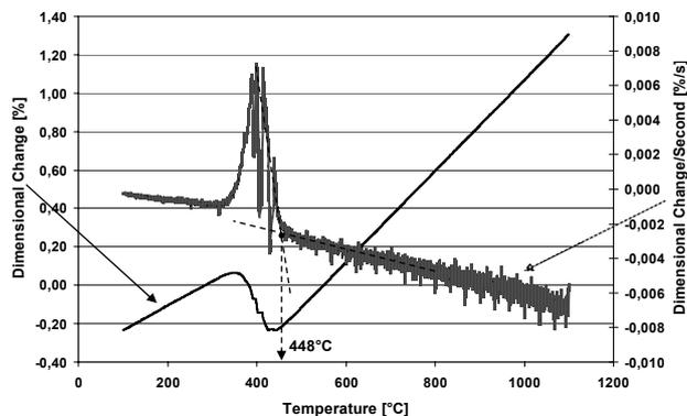
**Fig. 1. Detection of a transformation (austenite to bainite) by observing the dimensional change per second: Start of the transformation at 448°C.**
