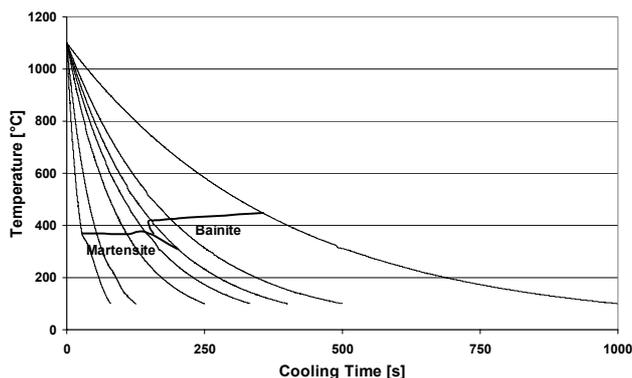
**Fig. 2. CCT diagram of the examined material.**
