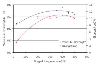
Fig. 2. Influence of forging temperature on tensile strength and elongation for sinterforged AX 431 Nr.10490
