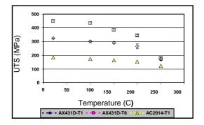
Fig. 1. Elevated temp.tensile testing for AX 431 Nr .10490 MPa –bars ,as sintered, for both T1 and T6 condition. (4)
