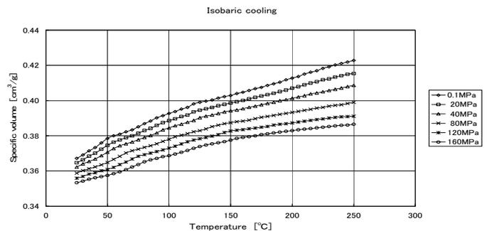
**Fig. 1. PVTgraph measured by material property tests.**
