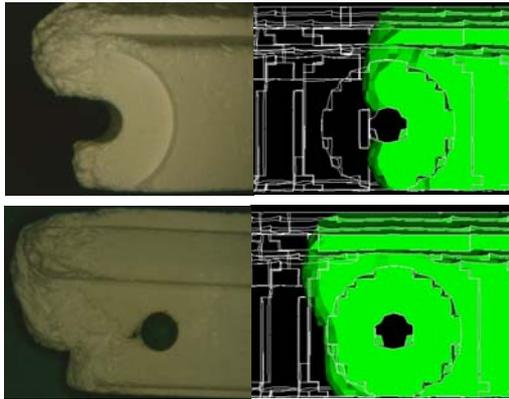
**Fig. 2. Comparison with experiment and simulation results about flow pattern around hole for pin.**
