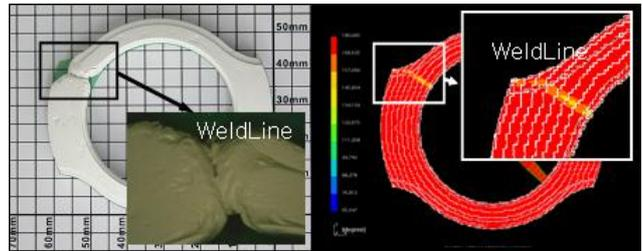
**Fig. 3. Weld line location by experiment(left) and weld line location predicted by simulation(right).**
