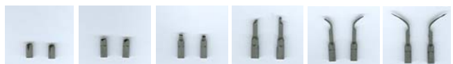
Fig. 4. Short shot experiment of dental scaler tip using the PIM feedstock (STS316L).
