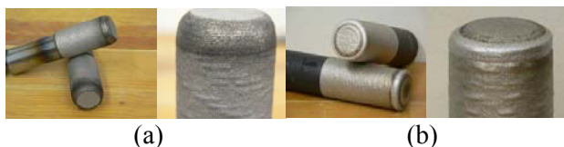
Fig. 2. Extrusion mandrel tools LPD clad with a) NiTung-60 and b) CCW-plus.
