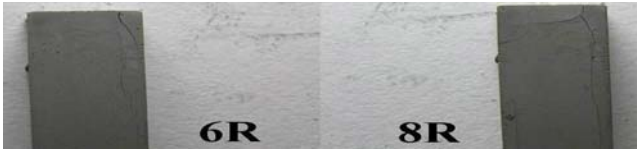
Fig. 2. The surface of the specimens that used feedstocks recycled 6 and 8 times after solvent debinding, showing more defects in the 8R specimen.
