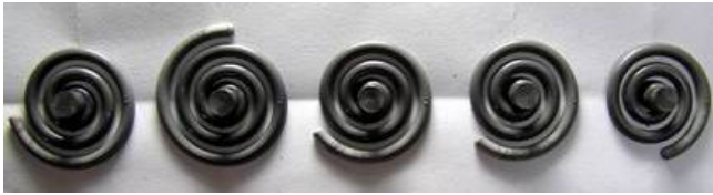
Fig. 1. Spiral flow length of the specimens of 0R, 1R, 3R, 6R and 8R (from left to right)
