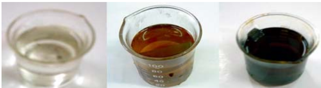
Fig. 3. The heptane color after solvent debinding for pure soluble binder, 0R, and 8R specimens. (From left to right)
