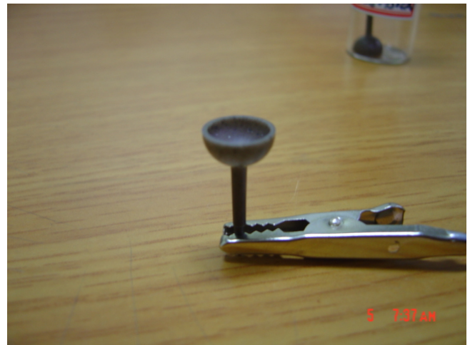
Fig. 3. A photo of a contaminated arc-tube
