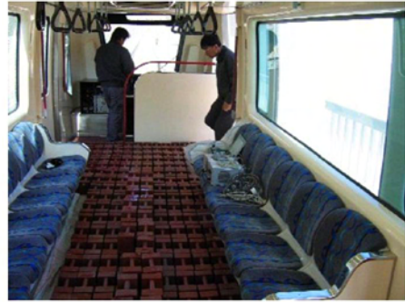
Fig. 2 Maximum weight condition of the rubber-tired vehicle
