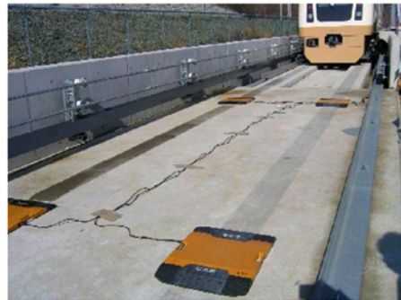
Fig. 3 Measurement of maximum wheel loads of the rubber-tired vehicle
