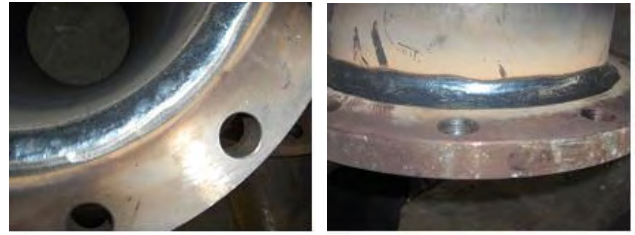
Fig. 7 Welding part of bell-mouth
