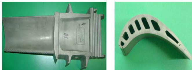
Fig 1. 1'st stage bucket of GE 7FA+e type gas turbine (left side)
