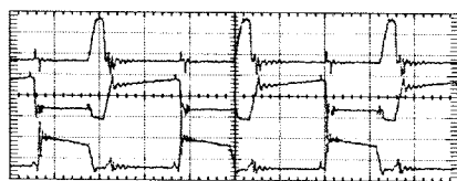
(b) CH3( I_{sa} ) : 5[A/div], CH5( I_s ) : 5[A/div], CH6( I_d ) : 5[A/div]
