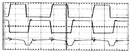
(c) CH2( V_{ds} ) : 100[V/div], CH1( V_{gs} ) : 100[V/div], CH3( I_s ) : 5[A/div]
