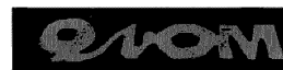
Figure 3. Fluorescence patterned image through photomask on a silicon wafer by UV irradiation for 10 min (spin-coated from 1 wt% chloroform solution without PAG).
