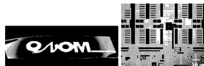
Figure 2. Fluorescence patterned image through a photomask on a glass slide by UV irradiation for 30 min (left) and on a silicon wafer by UV irradiation for 10 min (right). Polymer film was spin-cast from 1 wt % chloroform solution without PAG. Green fluorescence portion was unexposed to UV.
