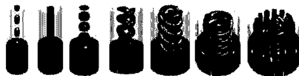
Figure 2. The simulated morphologies of asymmetric block copolymer in cylindrical pore with different pore diameter. The surface attracts minor A-block. Only A-domains are represented.
