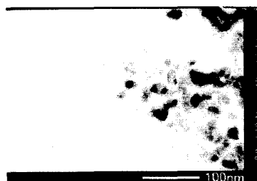
Fig. 6 TEM image of the plasma-treated TiO 2 film
