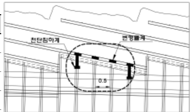
Fig.1 Details of Installation of Instruments
