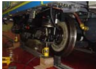
Figure 4 Hydraulic cylinder and packer
