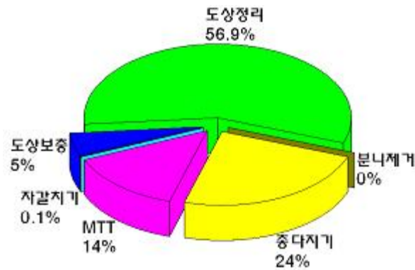
Fig 22. A state of ballast repair
