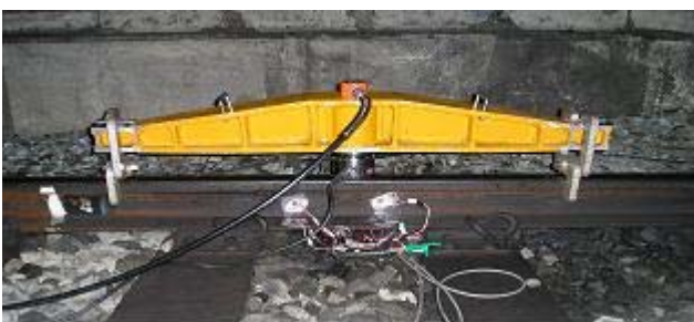
Fig 7. View of the test of the load calibration
