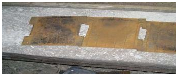
Fig 18. View of rail pad on the field test
