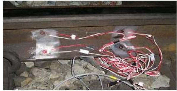
Fig. 3 Sight of the attachment of sensors
