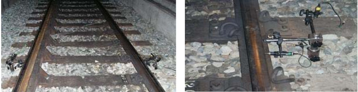
Fig 7. Sight of the attachment of LVDT
