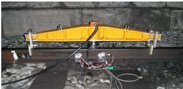
Fig. 4 View of the test of the load calibration
