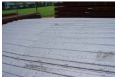
Fig.8 The appearance of deformed panel
