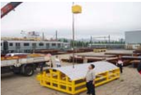
Fig.7 Weight drop test
