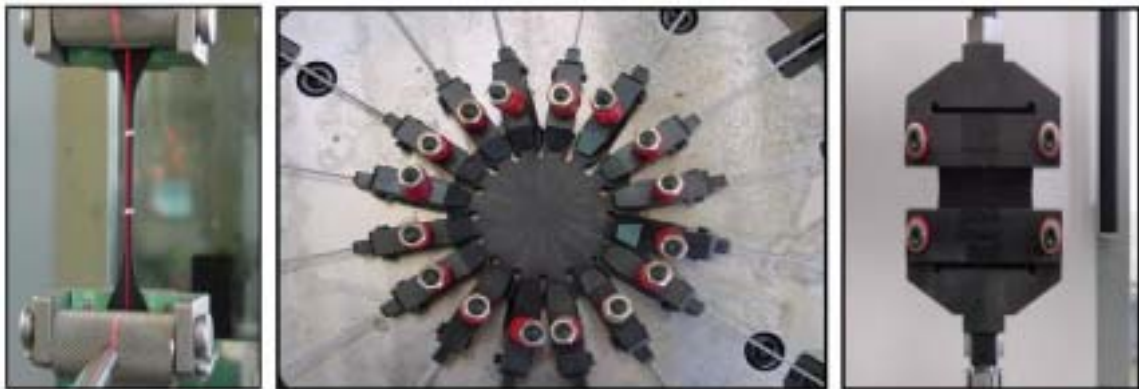
(a) Simple tension (b) Equi-biaxial tension (c) Pure shear
