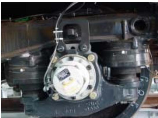
Fig. 5 Telemeter mounting on the axle box
