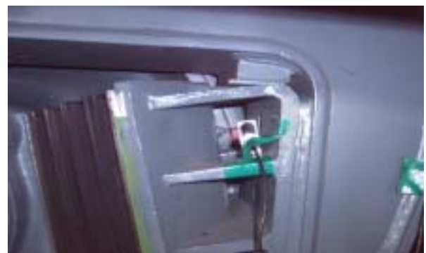
Fig. 6 Installation of tachometer sensor on a passenger bogie
