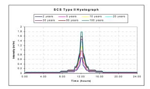
Figure 3. SCS Type II hyetographs of 2 to 100-year return period for Ulsan-Hwabong Watershed
