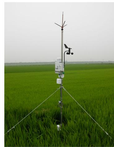
Fig. 2 Meteorological measurement equipment in study areas
